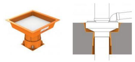
Where there is limited ceiling space and so the plastic pipe can be installed closer to the ceiling with the pipe connection recessed in the slab. When installing the QuelCast Manifold on the underside of the floor slab, ensure that you cut off the spigot on the manifold and then, using self-tapping steel screws, secure the QuelCast110 Cast In Fire Collar to the manifold.
